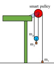
A mass  $m_1$  (60 grams) sitting on the floor is attached to a string that is threaded up and over a Smart Pulley. The string runs down the other side to and a secondary, massive hanging pulley (mass  $m_p$  --you'll have to
